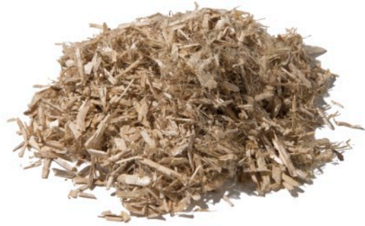
Loose fill hemp hurd. Different grades and consistencies of hurd are available.
